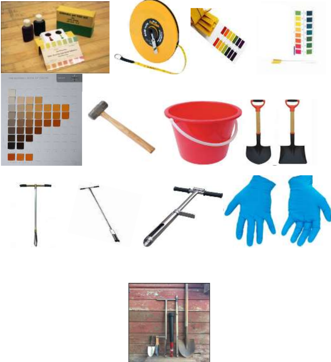
Fig: 1.1 tools and equipment needed for soil sampling and testing
